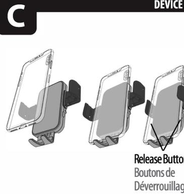
With the device holder plugged into power, the arms will open up automatically when a phone is not detected. When a Qi-enabled phone is detected, the arms will close automatically.
